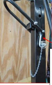
Note position of lifting hooks assembled on inside edges of "U" lifting lever
