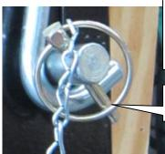
Lynch Pin fitted correctly
